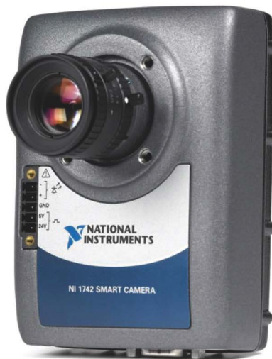
Figure 2 The NI 1742 smart camera includes an image sensor, a processor, and vision-analysis software to return inspection results instead of images.
