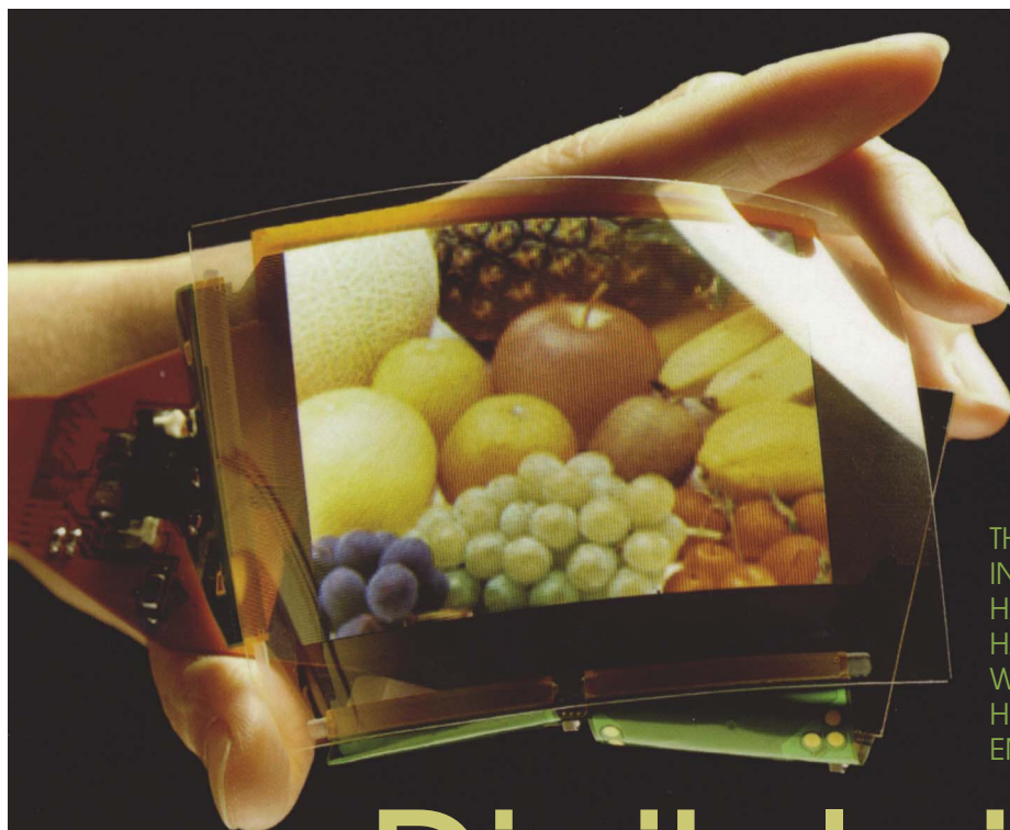
Figure 1 Sony is producing a lightweight and flexible full-color display by depositing an organic TFT directly onto a plastic substrate.
